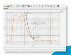
Advanced functions and graphical tools include crop, markers, zoom and graph annotation. In addition, sophisticated data analysis functions enable users to perform derivative and regression functions, as well as view comprehensive statistics.
